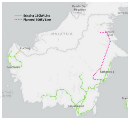
Figure 5.4-5 Outline of the 500kV backbone in Kalimantan
